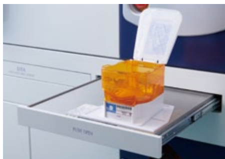
The cassette is recognized with RFID. (PET.P)
