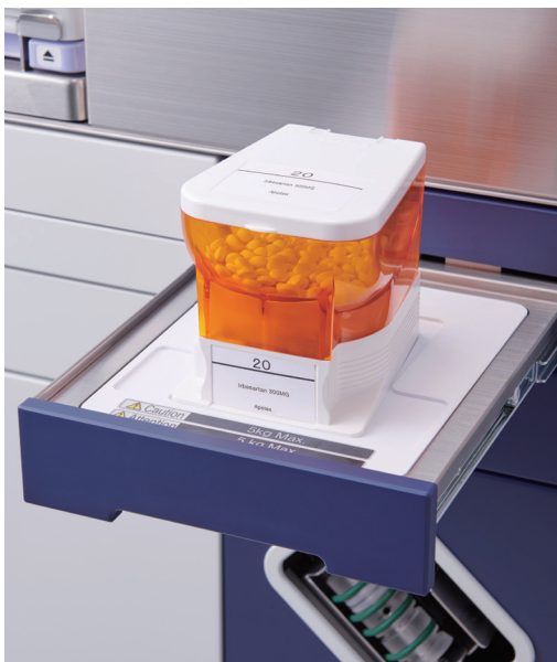
RFID recognizes the canister
